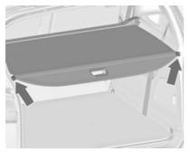
Pull the load compartment cover towards the rear using the handle and engage it in the retainers at the sides.
