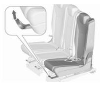
When using ISOFIX fastened child restraint systems on the second seat row, we recommend to adjust the accordant outer seat in third notch from rear end position, regarding to base seats. Lounge seat, if equipped, must be in normal position  $\diamondsuit$  44.
