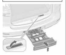
Push the release lever up and hold. Lift the rear carrier system slightly and push it into the bumper until it engages.
