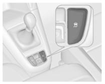
TC can be switched off when spinning of drive wheels is required: press  $\mathfrak{B}$  briefly.
