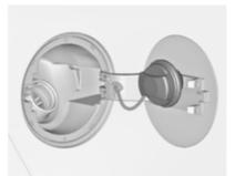
The fuel filler cap can be retained in the bracket on the fuel filler flap.
