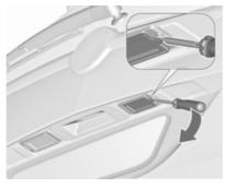
1. Insert screwdriver in recess of the cover, press to the side and release spring. Remove cover.
