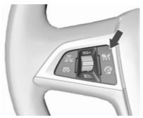
Press % to switch on adaptive cruise control. The control indicator (5) illuminates white. Additionally % appears in the Driver Information Centre.
