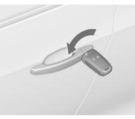
Manually unlock the driver's door by turning the key in the lock. Switch on the ignition and press to unlock all doors, load compartment and fuel filler flap. By switching on the ignition, the anti-theft locking system is deactivated.
