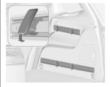
Insert the hook in the desired position first in the upper groove of the rail and then press in the lower groove. To remove, first pull out of the upper groove.
