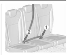
Remove lower latch plate from retainer and click it into left-hand buckle (1) at the centre seat. Guide the upper latch plate with the belt over the lap area and the shoulder (do not twist) and click into right-hand buckle (2) at centre seat.
