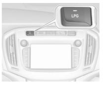
Press **LPG** to switch between petrol and liquid gas operation. The LED — status shows the current operating mode.
