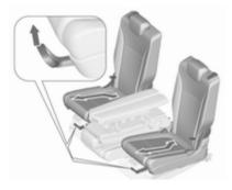
In lounge position, the outer seats are additionally movable in transverse direction when the centre seat backrest is folded to an armrest.
