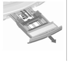
Completely pull out the rear carrier system until you hear it engage.
