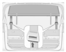
Push button on the tightener to release the strap on both sides. Detach hooks from the eyes. Unhook the safety net rods from the brackets in the roof frame. Roll up the net and secure with a strap.
