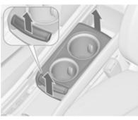
Pull the handle in front of cupholder and remove it vertically out of the console.
