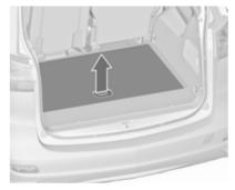
On versions without third seat row, there are storage boxes under the floor cover. To open lift up the cover and fold it upright behind rear seats.
