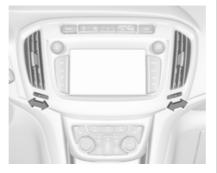
To open the vent, turn the adjuster wheel to I. Adjust the air amount at the vent outlet by turning the adjuster wheel.
