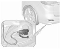
1. Turn the bulb socket anticlockwise and remove it from the reflector.
