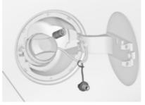
Screw the required adapter hand-tight onto the filler neck.
