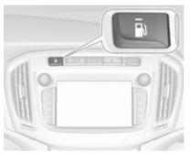
Press to switch between petrol and natural gas operation. The LED — status shows the current operating mode.
