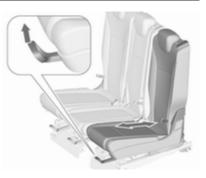
Pull handle, slide seat, release handle and allow seat to engage.
