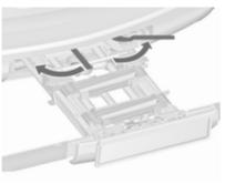
Swivel both clamping levers sideways as far as they will go. Otherwise safe functionality is not guaranteed. Fold out wheel recesses
