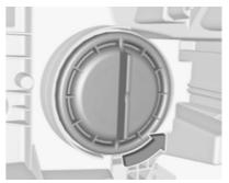
1. Rotate cap anticlockwise and remove it.
