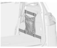
Insert adapters into the required position in the rails. The net pocket can be suspended from the adapters.
