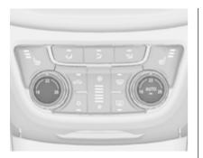
If the minimum temperature **Lo** is set, the climate control system runs at maximum cooling, if cooling 🗱 is switched on.
