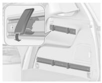
Install the hooks in the desired position in the rails: insert the hook in the upper groove on the rail and press in the lower groove. Lashing eyes
