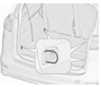
The lashing eyes are designed to secure items against slippage, e.g. using lashing straps or luggage net.
