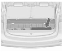
Stow the warning triangle in the storage of the load compartment floor in front of the tailgate.
