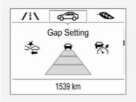
If Adaptive cruise control is active, this page shows the alert sensitivity setting instead of following distance setting. ♀ 176.
