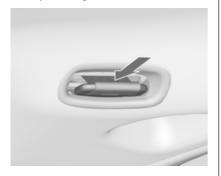
Insert in the seat belt holder in the roof with the lower latch plate pointing forward.
