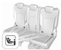
Fasten vehicle-approved ISOFIX child restraint systems to the ISOFIX mounting brackets. Specific vehicle ISOFIX child restraint system positions are marked in the ISOFIX table  $\Rightarrow$  63.
