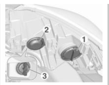
Low beam (1) outer bulb. High beam (2) inner bulb. Front turn signal light (3)
