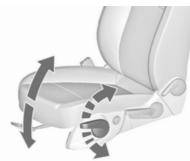
Lever pumping motion up : front end higher down : front end lower
