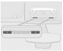
Operated by pressing ☆ and ☆ in front and rear courtesy lights.
