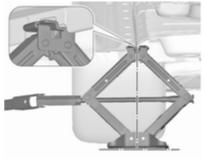
5. Set the jack to the necessary height. Position it directly below the jacking point in a manner that prevents it from slipping.
