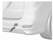
Insert a screwdriver in the slot at the lower edge of the cap. Release the cap by carefully moving the screwdriver downwards. To prevent damage it is recommended to place a cloth between the screwdriver and the frame.
