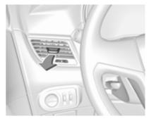
To close the vent, turn the adjuster wheel to  $\ensuremath{\textbf{0}}$  .
