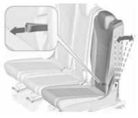
Raise backrest to vertical position. Adjust inclination by pulling the loop.
