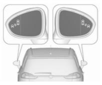
Side blind spot alert is active from speeds of 10 km/h up to 140 km/h. Driving faster than 140 km/h deactivates the system, indicated by low lighting warning symbols  $\alpha^{\text{ef}}$  in both exterior mirrors. Reducing the speed again will extinguish the
