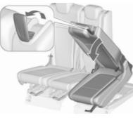
Folding back easy entry First move seat to desired position and then raise backrest.
