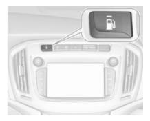
Pressing Switches between petrol and natural gas operation. Switching is not possible at high loads (e.g. powerful acceleration, driving at full throttle). The LED status shows the current operating mode.
