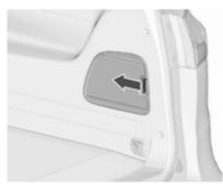
To open, release cover in side trim panel and remove.
