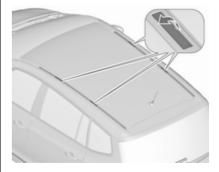
To fasten a roof rack, open the caps in the roof strips. Insert the mounting provisions, as instructed, in the retainer indicated in the illustration.
