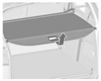
Remove load compartment cover from side brackets. Hold the handle and guide the load compartment cover until it is fully rolled up.
