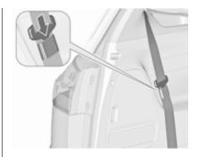
Before operating the load compartment cover, insert the latch plate of the seat belt on each side into the pocket that is mounted at the belt.
