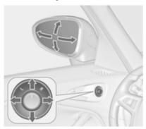
Select the relevant exterior mirror by turning the control to left (L) or right (R). Adjust respective mirror by tilting the four-way control.
