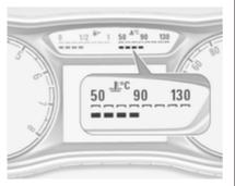
Number of LEDs displayed shows the coolant temperature.
