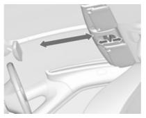
Pull the slider to open the cover of the panorama roof.
