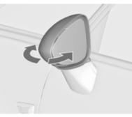
For pedestrian safety, the exterior mirrors will swing out of their normal mounting position if they are struck with sufficient force. Reposition the mirror by applying slight pressure to the mirror housing.
