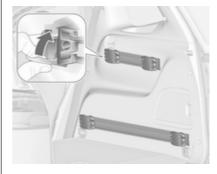
Fold open the handle plate, insert the adapter into the upper and lower groove of the rail and move to the required position. Turn the handle plate upwards to lock the adapter. To remove, turn the handle plate down and move out of the rail.
