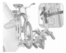
4. Guide the strap attached to the adapter underneath the lever to fold back the rear carrier system. Fasten the strap.
