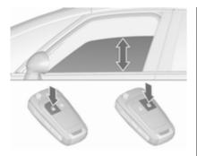
Press and hold to open windows. Press and hold to close windows. Release button to stop window movement.
