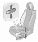
Move switch upwards/downwards.
