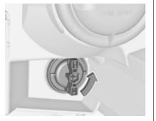
1. Rotate bulb socket anticlockwise to disengage. Withdraw the bulb socket from the reflector housing.
