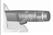
Pull lever. Washer fluid is sprayed onto the windscreen and the wiper wipes a few times.
