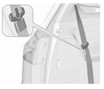
When seat belts are not used or when folding the seats, insert the latch plate of the seat belt on each side into the pocket that is mounted at the belt.
