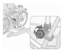
2. Attach the short mounting bracket to the bicycle frame. Turn the knob clockwise to fasten.
