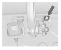
Attach breakaway stopping cable to eye.
