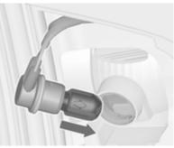
3. Remove the bulb from the socket by pulling.
