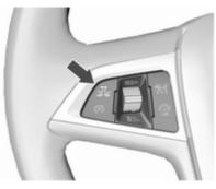
Press St; the current setting is shown in the Driver Information Centre. Press St again to change the alert sensitivity. The setting is also displayed in the top line of the Driver Information Centre.
