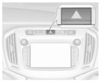
Operated by pressing ▲. In the event of an accident with airbag deployment the hazard warning flashers are activated automatically.
