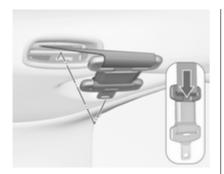
Push the top latch plate into the retainer. Fold over locked together latch plates against the seat belt.
