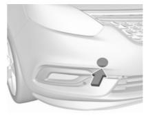
Disengage cap at bottom and remove downwards.
