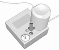
If the prescribed tyre pressure is not obtained within ten minutes, remove the tyre repair kit. Move the vehicle one tyre rotation. Reattach the tyre repair kit and continue the filling procedure for ten minutes. If the prescribed tyre pressure is still not obtained, the tyre is too badly damaged. Seek the assistance of a workshop. Drain excess tyre pressure with the button over the pressure indicator.
