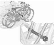
Use the short accessory mounting bracket to attach the fourth bicycle. The bracket must be fixed between the frames of the third and fourth bicycle.
