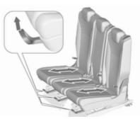
In normal position, the three seats of the second seat row can be individually moved in longitudinal direction.
