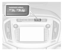
If the control indicator ON  $\Re_2$ illuminates for approx. 60 seconds after the ignition is switched on, the front passenger airbag system will inflate in the event of a collision.
