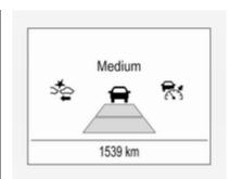
The selected following distance is indicated by filled distance bars on the adaptive cruise control page.
