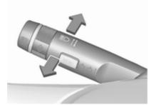
headlight flash : pull lever high beam : push lever low beam : push or pull lever
