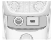
A 12 Volt power outlet is located in the front console. Fold the cover downwards.
