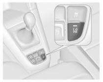
The lane departure warning system is activated by pressing lat. The illuminated LED in the button indicates that the system is switched on. When the control indicator lat in the instrument cluster illuminates green, the system is ready to operate.
