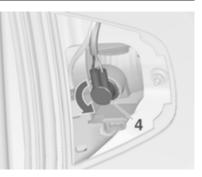
2. Turn the bulb holder anticlockwise and remove it from the reflector.
