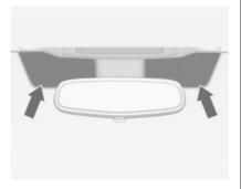
The marked areas on the windscreen are not covered with the coating. Devices for electronic data recording and fee payment must be attached in these areas. Otherwise data recording malfunctions may occur.
