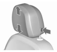
Press release button, adjust height, engage.
