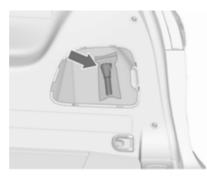
The funnel is located on the right side storage in the load compartment.
