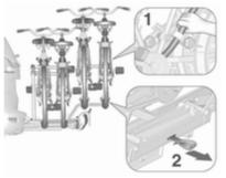
Hold frame (1) of rearmost bicycle with one hand and pull the loop (2) to disengage.
