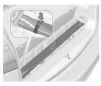
Fasten the load compartment cover in the storage with the Velcro tape.
