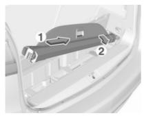
Insert the load compartment cover into the opening on the right side of the storage (1) and turn it until the handle rests flat on the housing (2).
