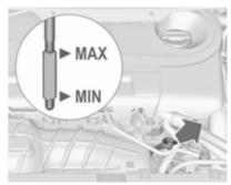
When the engine oil level has dropped to the **MIN** mark, top-up engine oil.
