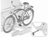
1. Rotate the pedals into position as shown in the illustration and put the bicycle on the foremost wheel recess.
