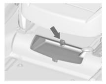
There is a storage box under the passenger's seat. Slide the rollo to open or close the box. Maximum load: 1.5 kg.
