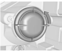
1. Rotate cap anticlockwise and remove it.
