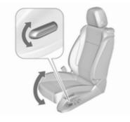
Move front of switch upwards/ downwards.
