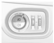
Operated by pressing ≢D. Light switch in position **AUTO**: switching on front fog lights will switch headlights on automatically.
