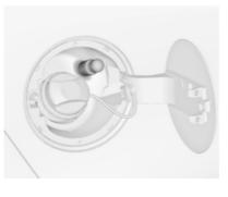
The fuel filler flap can only be opened if the vehicle is unlocked. Release the fuel filler flap by pushing the flap.
