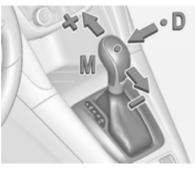
Move selector lever out of position  ${\bf D}$  towards the left in position  ${\bf M}$ .
