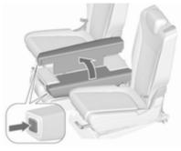
Push the left and right buttons near the centre head restraint and fold in the outer backrest parts, to be used as an armrest. Engage backrest parts in armrest position.
