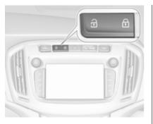
Press To lock. Press To unlock. Fault in radio remote control system
