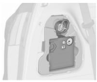
If equipped with tyre repair kit, remove the complete box.
