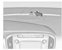
Status LED is integrated into the sensor on top of the instrument panel.
