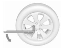
2. Fold out the wheel wrench and install ensuring that it locates securely and loosen each wheel nut by half a turn.
