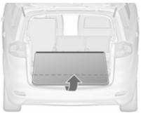
• Pull out the mat a little to protect load compartment sill when loading heavy objects. Raise up the overlaying part of the mat before closing the tailgate. Covering the load compartment up to the backrests of the front seats Only possible with Flex cover interior protection mat being folded at the zipper to half size (double layer).
