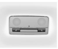
Illuminate in conjunction with the front courtesy light depending on rocker switch position.
