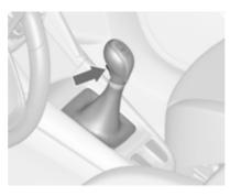
To engage reverse, depress the clutch pedal and then press the release button on the selector lever and engage the gear.
