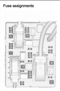
No. Circuit 2 Trailer outlet 3 Parking assist 4 Selective catalytic reduction system 5 6 7 Power seat 8 9 Selective catalytic reduction system 10 Nitrogen oxide sensor Trailer module/Trailer socket 11 12 Trailer module
