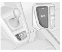
Deactivate the stop-start system manually by pressing **eco**. The deactivation is indicated when the LED in the button extinguishes.
