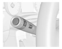
Select Vehicle Information Menu 🖘 by pressing **MENU** on the turn signal lever. Turn the adjuster wheel to select **Remaining Oil Life**.
