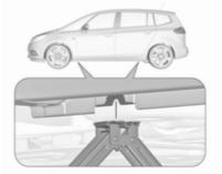
4. Ensure the jack is correctly positioned under the relevant vehicle jacking point.
