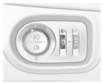
To adapt headlight range to the vehicle load to prevent dazzling: turn thumb wheel <sup>€</sup> to required position.
