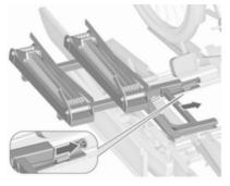
1. Attach the adapter to the rear carrier system as shown in the illustration.
