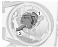
2. Rotate the bulb holder anticlockwise to disengage. Withdraw the bulb holder from the reflector housing.
