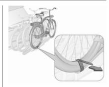
Additionally secure both bicycle wheels of the fourth bicycle to the wheel recesses using the tensioning straps.
