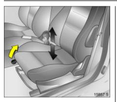
Adjusting the seat height Lift lever and relieve some weight from seat to raise it or press down on seat with body weight to lower it.
