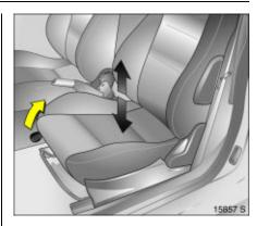
Seat cushion height: Pull lever Lift lever and relieve some weight from seat to raise it or press down on seat with body weight to lower it.
