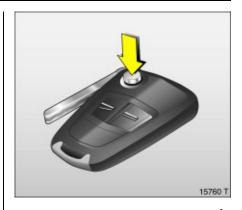
Key with retractable key blade \* Press button to extend. Press button to retract; key section engages audibly.
