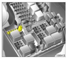
Place spare fuses at the point provided in the fuse box; next to this on the right is the fuse puller for changing fuses.
