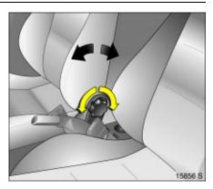
Adjusting the backrest Turn side handwheel on the seat while releasing the pressure on the backrest.
