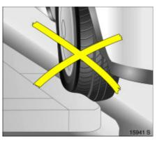
**Tyre condition, wheel condition** Drive over edges slowly and at right angles if possible. Driving over sharp edges can cause tyre and wheel damage. Do not trap tyres on the kerb when parking.
