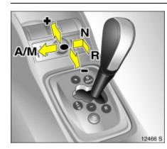
Selector lever in A/M Switch between Automatic and Manual mode.
