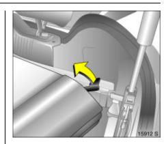
14. Release the roof retainer at the rear left of the luggage compartment partition by raising the release lever.
