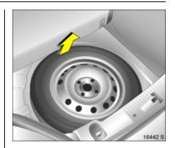
Pull the spare wheel forward and then upward out of the wheel well.
