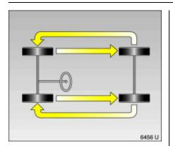
If wear is greater in the front than in the rear, switch the front and rear tyres. Correct tyre pressure.
