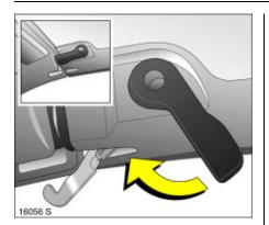
Push the locking levers on the right and left side of the window frame all the way up.
