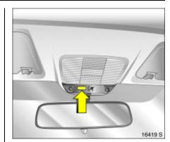
2. Press button in front of the courtesy lamp (with ignition off); LED in the hazard warning lamp button flashes a maximum of 10 seconds.
