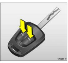
The remote control has a range of approx. 5 metres. This range can be affected by outside influences. Aim the remote control at the vehicle to operate. The hazard warning lamps flash to confirm remote control operation.
