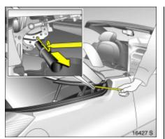
9. Use the tool to forcefully pull the lock bar to unlock the cover in front of the rear window. The lock bar is on the right side of the car below the cover.
