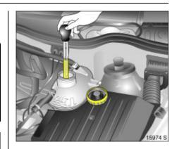
Antifreeze and corrosion protection Before the start of winter, have a workshop check the antifreeze protection. The antifreeze level must guarantee protection to approx. -28 C. Insufficient antifreeze will reduce the frost protection level and the corrosion protection. If necessary add antifreeze.
