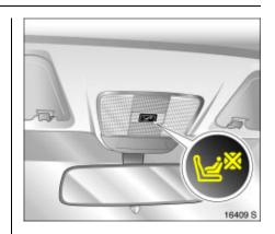
If the control indicator does not light during driving, the front and side airbags for the front seat passenger are not de-activated and there is a risk of fatal injury to the child. Have a workshop eliminate the cause of the fault.
