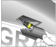
2. Rotate bulb holder to left and disengage.
