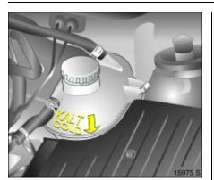
**Coolant level** In a closed cooling system, there is hardly any loss.
