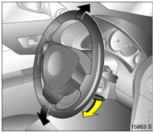
Steering wheel adjustment **\***: Swivel lever down, adjust height, swivel lever up, engage Adjust steering wheel only when vehicle is stationary and steering column lock is released.
