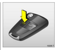
**Central locking system** Used to unlock and lock doors, luggage compartment cover and fuel flap.
