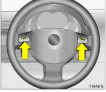
Horn:  $\blacktriangleright$  press right or left Airbag system  $\diamondsuit$  56, Remote control on steering wheel  $\divideontimes$   $\diamondsuit$  92.
