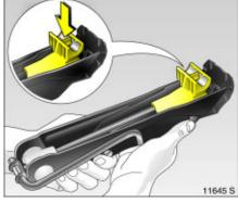
4. Set the jack \* to the necessary height. Position the jack arm at the front or rear so that the jack claw (arrow in Fig.) spans the vertical web and engages in the recess in the web. Make sure it is securely positioned.
