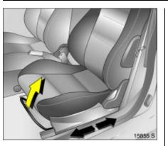
To adjust seat leg room: Pull handle, slide seat, release handle Seats  $\diamond$  46, Seat position  $\diamond$  47.
