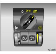
**Instrument illumination** Comes on with exterior driving lamps. Brightness can be adjusted with adjuster wheel.
