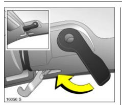
Move the locking levers on right and left of the window frames all the way up. Each retaining hook must engage and the roof must lock securely.
