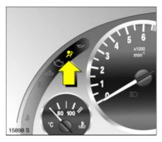
**Control indicator % for belt tensioners** The function of the belt tensioners and airbag systems is monitored electronically and indicated by the control indicator **%**. When the ignition is switched on, the control indicator illuminates for approx. 4 seconds. If it does not illuminate, or if it does not go out after 4 seconds, or if it illuminates whilst driving, there is a fault in the belt tensioner or airbag systems \$ 60. The systems might not trigger in the event of an accident.
