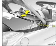
10. With the lock bar pulled, have a helper pivot the cover upward by hand. The noise arising from this is normal.
