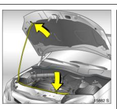
Secure the bonnet support. Before closing the bonnet, press the support into the holder.
