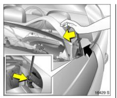
12. Release the front catches of the boot lid using the tool by inserting the tool in the guide and pressing the upper end inward; see figure. At the same time, pull the boot lid slightly upward out of the catch. Carry out the procedure on the right and left.
