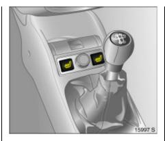
Heated seats ☆ Two pushbuttons ⊮ in the centre console. For heating with ignition on, press button ⊮.
