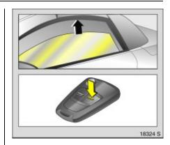
**Closing windows from outside** Press button — on the remote control until the windows are fully closed.
