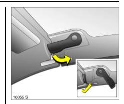
Release the locking levers on upper right and left of the window frames, pulling both levers all the way down. Both retaining hooks must unhook.
