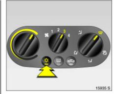
**To clear fogged or icy windows** Rotary knob for temperature and air mixture clockwise, air distribution on **W**, Air conditioning system **\*** : also press button **\$**
