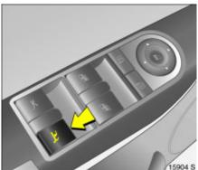
**Closing the roof** Only with stationary vehicle and closed boot lid.
