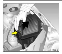
**Fuse box** The fuse box is located in the engine compartment next to the coolant expansion tank.
