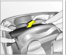
15. With the aid of a second person, carefully and slowly pull the roof upward. Grip the roof at the sides and pull forward. Make sure that the boot lid is completely open.
