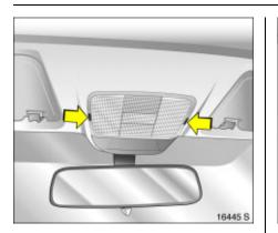
**Courtesy light** Front courtesy lamp 1. Unclip the scatter disc on the housing at
