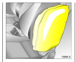
When deployed, the side airbag inflates within milliseconds and forms a safety cushion for the driver or front passenger in the respective front door area. This substantially reduces the risk of injury to the upper body and pelvis in the event of a side-on collision.
