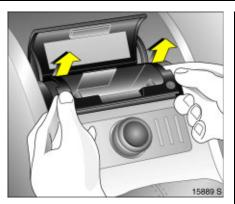
To empty, open the ashtray cover fully beyond its resistance point, causing the insert to lift. Grip both sides of the ashtray insert and pull upwards.
