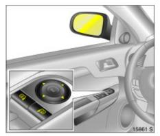
Adjust exterior mirrors Select corresponding exterior mirror and adjust with the four-way switch.
