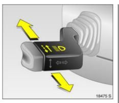
Headlamp flash, main beam and<br/>dipped beamHeadlamp flash=Pull stalk towards<br/>steering wheelMain beam=Push stalk forwardsDipped beam=Push stalk forwards<br/>again
