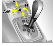
Operating the manual transmission automated with the selector lever Always move the selector lever all the way to the stop. Note the gear or mode indicator in the transmission display.
