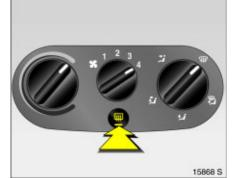
Heated rear window, heated exterior mirrors Operated with the III button.
