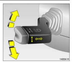
Switch on turn signal lamps
