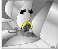
To adjust seat backrests: Turn handwheel Do not lean on seat backrest whilst adjusting it.
