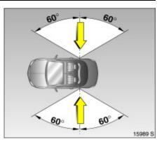
The side airbag system will be triggered:
