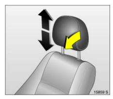
Head restraints Adjustment Tilt head restraints forwards, hold and adjust height. Allow head restraints to engage after adjustment.
