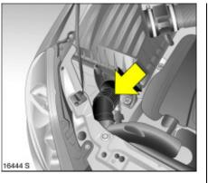
When replacing bulbs in the front right headlamp, detach the air hose from the air filter.
