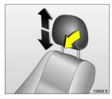
Head restraint height: To release, tilt head restraint forward, hold and adjust height, engage Head restraints \$\dot 48, Head restraint position \$\dot 49, Head restraint removal \$\dot 49.
