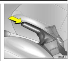
Releasing the hand brake: Raise lever slightly, Press release button, Lower lever fully Hand brake \$ 123.
