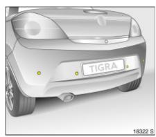
**Ultrasonic parking sensors \*** When reverse gear is selected, the park pilot switches itself on automatically.
