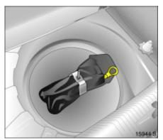
The towing eye is in the pouch or the stowage compartment for vehicle tools  $\diamondsuit$  135. Spare wheel  $\diamondsuit$  133.
