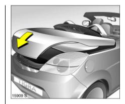
11. Press the button below the luggage compartment lid until the lid is completely closed.⇔ 28
