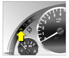
$\frac{\text{Control indicator } \checkmark b \text{ for engine electronics}}{\text{Comes on for a few seconds after the ignition is turned on.}}$
