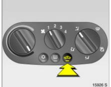
Air recirculation system বহু The air recirculation mode of the ventilation system is activated and deactivated by pressing the বহু button.
