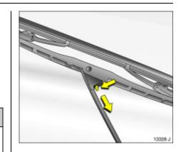
Windscreen wiper replacement Lift wiper arm. Move release lever and detach wiper blade.
