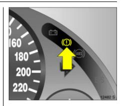
Brake system control indicator (D) The warning lamp lights up after the ignition is turned on, when the handbrake is applied or if the brake or clutch fluid level is too low. Brake fluid  $\diamondsuit$  168.
