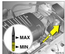
Pull out the dipstick, wipe it clean, insert it to the stop on the handle, pull out and read the engine oil level.
