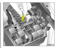
Slot fuse-gripping tool onto fuse and withdraw it.
