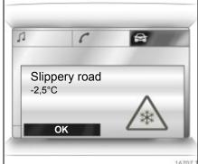
In vehicles with graphical information display \*, the warning message **Slippery road** is shown in the display as a warning for icy road surfaces. No message is displayed at temperatures below -5 C.
