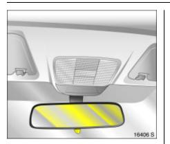
To adjust interior mirror by swivelling Swivel lever on underside of mirror housing to reduce dazzle. Interior mirror \$ 34
