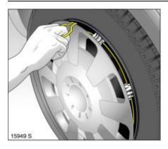
1. Pull off the wheel trim with the hook  $\stackrel{\textbf{*}}{\star}$ . Vehicle tools  $\stackrel{\textbf{\circ}}{\vee}$  135.
