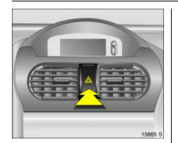
Hazard warning lamps Operated with the A button. Hazard warning flashers \$ 90.
