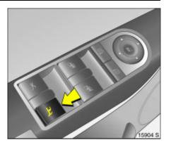
■ Press → until the roof and boot lid are completely closed.
