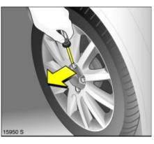
Alloy wheels \*: Prise off the hub cap \* with a screwdriver. Protect the rim by placing a soft cloth between the screwdriver and the alloy wheel.
