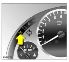
**Control indicator for immobilizer** 《칭 Control indicator 《칭 illuminates briefly when the ignition is switched on.
