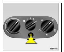
Heated exterior mirrors \* Heating is activated or deactivated by pressing the IIII button when the ignition is on.
