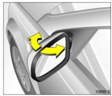
Swinging in exterior mirror The exterior mirrors can be folded in by pressing gently on the outer edge of the housing.
