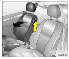
Fold backrest forward To fold the backrest forwards, – e.g. to reach the storage compartment behind the seats, – lift release lever.
