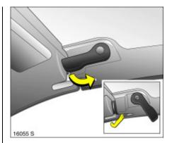
Release the locking levers on upper right and left of the window frames, pulling both levers all the way down. The retaining hook must unhook.
