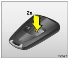
If the ignition was switched on, the driver's door must be opened and closed once so that the anti-theft alarm system can be switched on.
