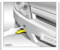
**Towing your own vehicle** Disengage cap at bottom and remove downwards.
