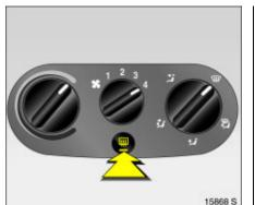
Heated rear window Heating is activated or deactivated by pressing the IIII button when the ignition is on.
