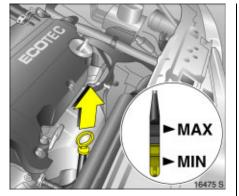
Check with the vehicle on a level surface. The engine must be at operating temperature and switched off for at least 5 minutes.
