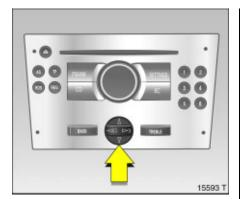
**To select with four-way button** Select menu items via menus and with the buttons/four-way button of the Infotainment system.
