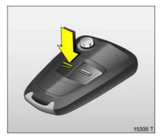
To deactivate Press button  $\geq$  of the radio remote control
