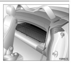
Stowage compartments Stowage compartment behind the seats The compartment is only suitable for stowing light objects. Maximum load: 10 kg.
