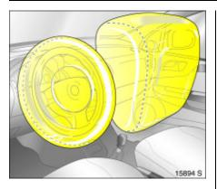
When triggered, the front airbags inflate in milliseconds and form a safety cushion for driver and front passenger. Forward movement is checked and the risk of injuries to the upper body and head thereby substantially reduced.
