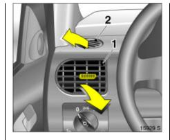
To close the vents, push the slider towards the centre of the vehicle.
