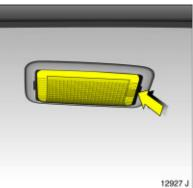
**Luggage compartment lamp** 1. Prise the lamp out with a screwdriver.
