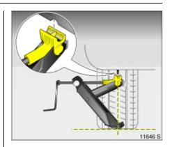
The edge of the jack base must be on the ground directly below the jacking point in a manner that prevents it from slipping.
