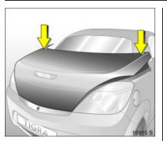
Have a second person help to force the boot lid closed simultaneously on the right and left. It must engage in the locks.
