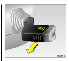
**Windscreen washer system** Pull stalk towards steering wheel. Washer fluid sprays onto the screen and the wipers are engaged for a few wipe movements.
