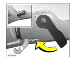
17. Push the locking levers on the right and left side of the window frame all the way up.
