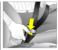
**Removing the belt** To release seat belt, press red button on belt buckle.
