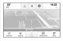
The current location is indicated by a circle with an arrow pointing into the direction of travel.
