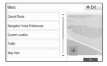
Select **Current Location** to display the respective submenu indicating details on the nearest address, the coordinates, and Points of interest (\$\phi\$ 49) around the current location.
