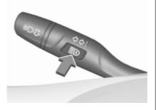
The green control indicator **E** illuminates continuously when the assist is activated, the blue one **E** illuminates when high beam is on. Control indicator **E** □ ♦ 102.
