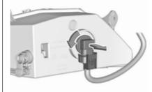
4. Turn the bulb socket anticlockwise and remove it from the light assembly.
