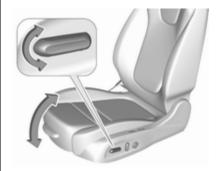
Tilt front of switch upwards/downwards.
