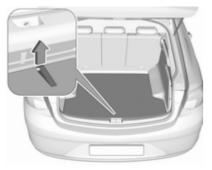
The rear floor cover can be removed. Raise cover at the loop and remove.
