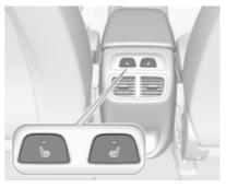
Activate seat heating by pressing #/ for the respective rear outer seat. Activation is indicated by the LED in the button.
