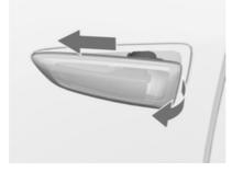
1. Slide lamp to its left side and remove with its right end.
