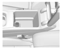
An USB port for charging devices is located below the foldable armrest. The USB port has also a data connection to the Infotainment system.
