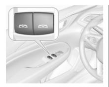
Operate And for the respective window by pushing to open or pulling to close.
