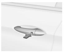
Electronic key system: Unlocking the vehicle by pressing the button on any exterior door handle deactivates the anti-theft alarm system.
