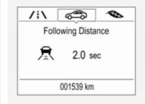
On Mid- and Uplevel display, select **Info** menu via steering wheel buttons and press **▼** to select following distance indication \$\dip\$ 104.
