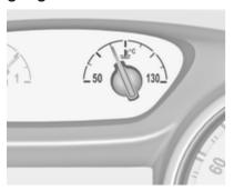
Displays the coolant temperature.
