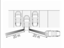
The system sensors cover a zone of approx. 20 metres at 90° to the left or right side behind the vehicle. Rear cross traffic alert is active up to 10 km/h and issues alerts within cross traffic travelling between 0 and 36 km/h.
