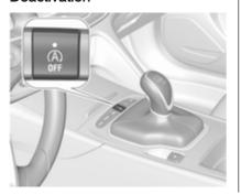
Deactivate the stop-start system manually by pressing a. Deactivation is indicated when the LED in the button illuminates.
