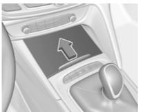
A storage box is located in the centre console. Push cover to the front.
