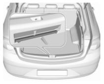
Stow the warning triangle in the space at the rear of the load compartment.
