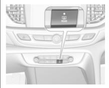
Operated by pressing a together with heated exterior mirrors. LED in button illuminates.
