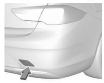
Disengage cap at bottom and remove downwards.
