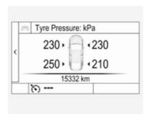
System status and pressure warnings are displayed by a message indicating the corresponding tyre in the Driver Information Centre.
