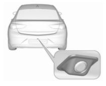
The camera is mounted between the number plate lights.
