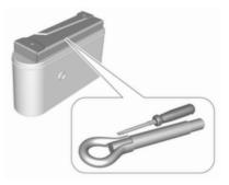
The tools and the towing eye are located in a box together with the tyre repair kit below the floor cover in the load compartment.
