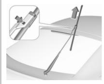
Lift the wiper arm until it stays in the raised position, press button to disengage the wiper blade and remove.
