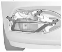
Undo three screws and remove the light assembly to the front.
