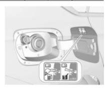
The misfuel inhibitor ensures that the flap of the fuel filler neck can only be opened by using the suitable fuel nozzle or a funnel for emergency refilling.
