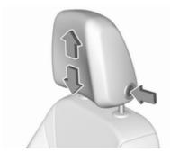
Press release button, adjust height, engage.
