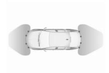
The system has four ultrasonic parking sensors each in the rear and front bumper.
