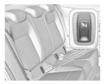
Fasten vehicle-approved ISOFIX child restraint systems to the ISOFIX brackets. Specific vehicle ISOFIX child restraint system positions are marked in the ISOFIX table ⋄ 62.
