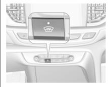
If the vehicle is equipped with heated windscreen, button  $\leftrightarrows$  is replaced by button  $\oiint$ .
