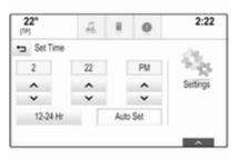
Select **Auto Set** at the bottom of the screen. Activate either **On - RDS** or **Off - Manual**.
