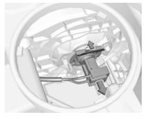
Disengage bulb holder by pressing the retainer to the front. Withdraw the bulb holder from the reflector housing.
