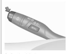
On Baselevel display press **SET/CLR** on the turn signal lever to confirm a message.
