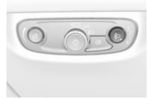
To adapt headlight range to the vehicle load to prevent dazzling: push and then turn to to required position.
