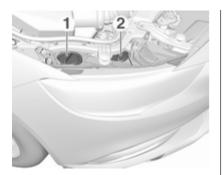
Low beam (1) outer bulb. High beam (2) inner bulb.
