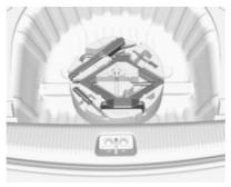
The jack with wheel wrench, the tools, an extension bolt for securing a damaged wheel and the towing eye are placed in the tool box below the spare wheel in the load compartment. Spare wheel ▷ 262.
