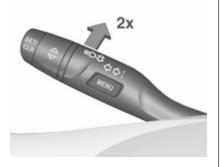
The high beam assist is activated by pushing the turn signal lever twice at a speed above 40 km/h.
