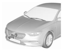
The radar unit is mounted behind the radiator grille behind or below the brand emblem.
