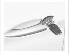
Manually unlock the driver's door by inserting and turning the key in the lock cylinder.
