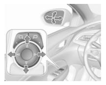
Select the relevant exterior mirror by pushing left or right mirror button. LED in button indicates the selection.
