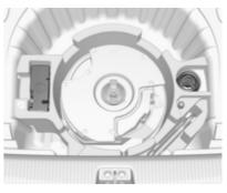
On vehicles with audio speaker system, the tyre repair kit is stowed together with the tools.
