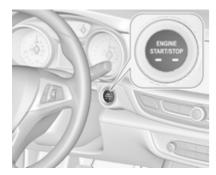
Electronic key must be inside the vehicle.
