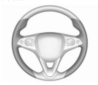
The recommended grip areas of the steering wheel are heated quicker and to a higher temperature than the other areas.
