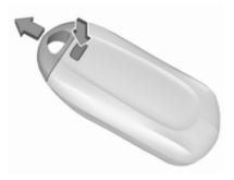
Press button at the back of the electronic key unit and extract the key blade from the housing.
