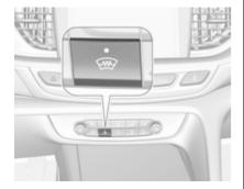
Operated by pressing . LED in button illuminates.
