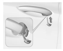
Electronic key: to remove the cap, press button at the back and extract the key blade from the housing. Insert the key into the recess at the bottom of the cap and swivel the key upward. Electronic key system ▷ 21.
