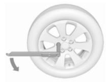
Fold out the wheel wrench and install ensuring that it locates securely and loosen each wheel nut by half a turn.
