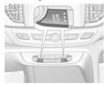
Adjust ventilation to the desired setting by pressing a for the respective seat one or more times. The control indicator in the button indicates the setting.
