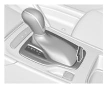
Release the selector lever trim from the centre console. Poke with a finger into the leather socket below the selector lever and push the trim upwards. Rotate trim to the left.
