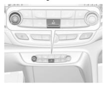
Press **A/C** to switch on cooling. Activation is indicated by the LED in the button. Cooling is only functional when the engine is running and climate control fan is switched on. Press A/C again to switch off cooling.
