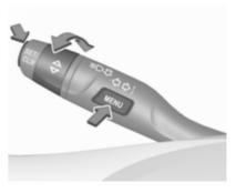
Press **MENU** to switch between the main menus or to return from a submenu to the next higher menu level.
