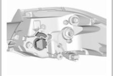
4. Turn the bulb carrier anticlockwise and remove it from the lamp assembly.
