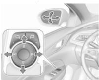
Select the relevant exterior mirror by pushing  $\square_i$  for left mirror or  $_i\square$  for right mirror. LED in button indicates the selection.
