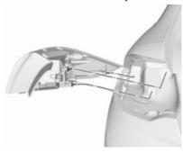
Carefully withdraw tail lamp assembly from recess and remove.
