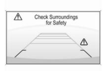
The area displayed by the camera is limited. The distance of the image that appears on the display differs from the actual distance.
