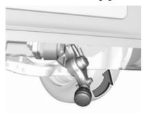
With the flat of the hand, swivel the released coupling ball bar to the right until it engages under the floor. Make sure that the release handle is back in its hidden initial position, otherwise the buzzing tone will not stop.
