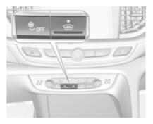
If the vehicle is equipped with heated windscreen, button **ON/OFF** is replaced by button .
