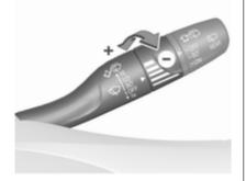
Wiper lever in position **INT**. Turn the adjuster wheel to adjust the wiping frequency.
