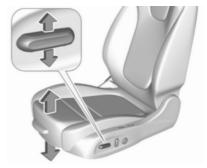
Move switch upwards/downwards.
