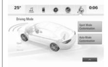
On 8" Info Display a Flex Ride visualisation menu can be displayed by touching & on the screen. On this page the selected drive mode and active setup are displayed.
