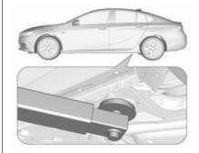
Rear arm position of the lifting platform at the underbody.
