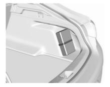
Stow the first aid kit on the right side of the load compartment and secure it with the strap.
