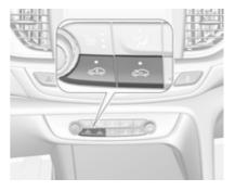
Press so to activate external air mode. LED is indicated.
