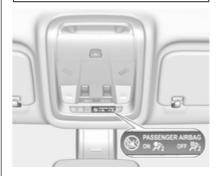
If the control indicator  $\aleph_2$  illuminates for approx. 60 seconds after the ignition is switched on, the front passenger airbag system will inflate in the event of a collision.
