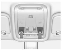
Operated by pressing the respective reading light.
