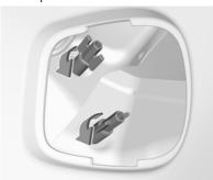
2. Unscrew the two plastic securing nuts from the inside by hand.
