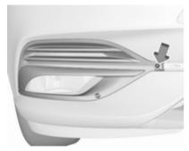
2. Undo screw and remove the faceplate.
