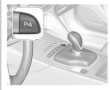
Press parking assist button P<sup>n/±</sup> to deactivate, the LED in the button extinguishes.
