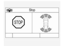
When a slot is detected, a visual feedback in the Driver Information Centre and an acoustic signal is given.
