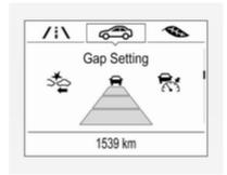
If Adaptive cruise control is active, this page shows the alert sensitivity setting instead of following distance setting. ▷ 181.
