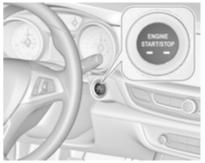
Power button: press **Engine Start/Stop** and release.
