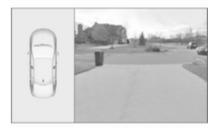
The screen in the Info Display is divided into two parts: on the left there is a view from above the vehicle, and on the right there is the view from front or the rear displayed, according to the gear engaged. The parking sensors complete the information on the view.
