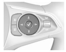
Press  $\triangleleft$  to open main menu page. Select a main menu page with  $\Delta$  or  $\nabla$ . Confirm a main menu page with  $\checkmark$ . Once a main menu page is selected, press  $\Delta$  or  $\nabla$  to select subpages. Press **▶** to open a next folder of the selected subpage.
