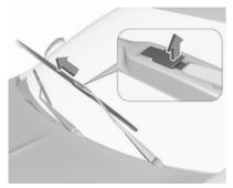
Lift the wiper arm until it stays in the raised position. Lift retaining clip to disengage the wiper blade and remove.
