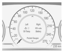
Press ► while pocket gauges is displayed. Select left or right pocket by pressing **⊳** or **⊲**. Choose gauge type for each pocket by pressing ∇. Confirm with **√**.
