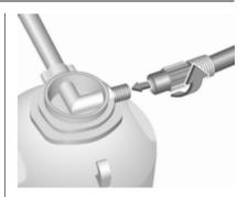
Type 1: screw the compressor air hose to the connection on the sealant bottle and fit the sealant bottle into the retainer on the compressor.
