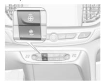
Press upper button \* to increase or lower button \* to decrease fan speed. The fan speed is indicated as pop-up in the Info Display. Fan speed can also be changed by touch buttons in the climate setting display. Press **Climate** to enter the menu.
