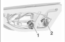
4. Turn the bulb carrier anticlockwise and remove it from the lamp assembly.
