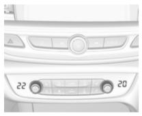
Set the preselected temperatures separately for driver and front passenger to the desired value using the left and right control dials. The knob on the passenger side changes the temperature for the passenger side. The knob on the driver's side changes the temperature for the driver's side or for both sides depending on activation of synchronisation **SYNC**. Recommended temperature is 22 °C.
