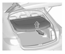
Lift cover at the rear and at the front. Remove the cover.
