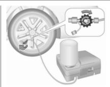
Type 2: remove protection cap from filler hose and screw the filler hose to the tyre valve. The air release valve must be closed (turn clockwise).
