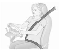
Pull out the seat belt and fasten in belt buckle. The seat belt must not be twisted and must fit close against the body. The backrest must not be tilted back too far (maximum approx. 25°).
