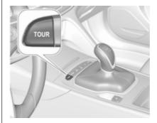
TOUR mode adjusts the settings of the systems for a comfortable driving style.
