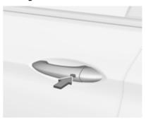
Press the button on any exterior door handle.
