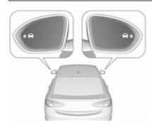
If the vehicle is equipped with lane change alert \$\phi\$ 207, the symbol ★ \$\epsilon\$ is displayed in the mirrors.
