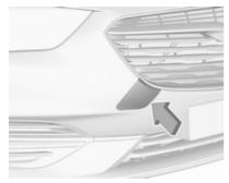
Disengage cap at slot and remove downwards.
