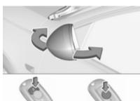
Press again after locking for one second to fold in mirrors.
