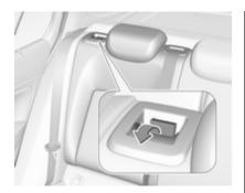
Pull the release lever on one or both outer sides and fold down the backrests onto the seat cushion. When folding the backrests, pull the seat belts along with them.
