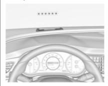
When approaching a detected pedestrian too quickly, a red flashing LED alert or the pop-up symbol  $\lambda$  in the head-up display is projected on the windscreen in the driver's field of view. A warning chime is provided. The brake system may prepare for driver braking to occur more rapidly which can cause a brief, mild deceleration. Continue to apply the brake pedal as required.
