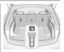
In addition to the ISOFIX brackets, fasten the Top-tether strap to the Top-tether fastening eyes.
