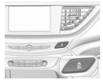
TC can be switched off when spinning of drive wheels is required: press \$\mathbb{g}\$ briefly.
