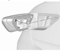
Carefully withdraw the lamp assembly from the recesses and remove.
