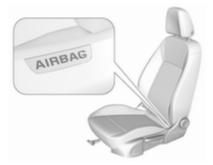
The side airbag system consists of an airbag in each front seat backrest and in the rear outboard seat backrests. This can be identified by the word AIRBAG.
