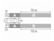
The system sensors cover a zone of approx. 3.5 metres parallel on both vehicle sides and approx. 3 metres rearwards on side blind zone alert (A) and approx. 70 metres rearwards on lane change alert (B) on parallel lanes. The zones start at each exterior mirror. The height of the zone is approx. between 0.5 metres and 2 metres off the ground.
